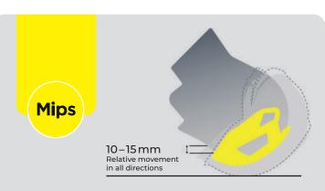
Mips is a low-friction layer inside the helmet. It is intended to reduce the rotational force to the head that is transmitted to the brain at impacts. The system allows for free movement of 10-15 mm between the helmet and the head in all directions. The Mips Brain Protection System is a Swedish patented solution based on over 20 years of studies by neurologists, bio-engineers and researchers at the Karolinska Institute and the Royal Institute of Technology.
